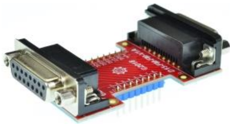
Figure 3: D15-F-F-V1A with headers
